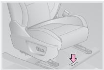
Vehicle Identification Number (VIN) is stamped under driver's seat.
