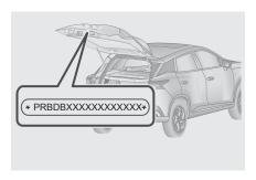
Vehicle Identification Number (VIN) label is located on back door as shown in the illustration.
